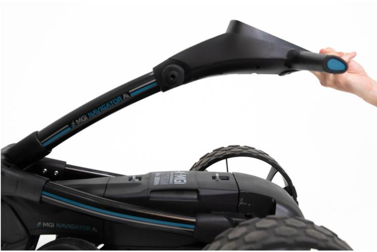
**STEP 3:** Lower handlebar until touching chassis.
