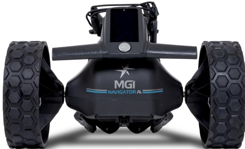
Press the black release button on the wheel hub. Place the wheel onto the axle. You will need to match up the inner female groove on the axle and the male of the wheel. See Section 3.3 for Rear Wheels Position.
