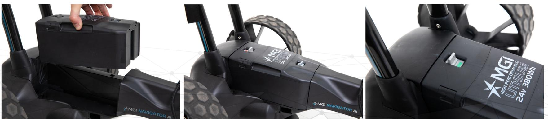
Your Ai Navigator GPS<sup>+</sup> has been equipped with a fail-safe battery connection, so the Ai Navigator GPS<sup>+</sup> will not move when you connect the battery. Your Ai Navigator GPS<sup>+</sup> will only start after the screen turns on. (Which may take up to 30 seconds). The Ai Navigator GPS<sup>+</sup> can then be activated by the speed control button or remote control.
