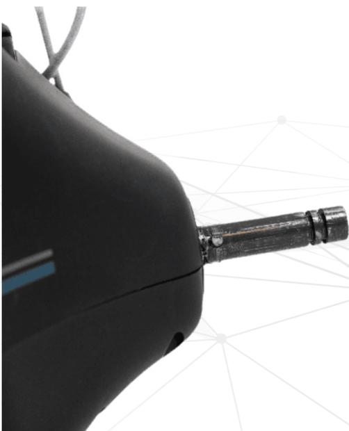
**i. Drive position** – Lock the wheel onto the groove closest to the battery base. To do this, press the black release button on the wheel hub, push the wheel onto the axle as far as possible and pull back until the wheel clicks into place. To test for drive position, try rolling the wheel backward.
