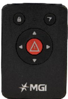
To turn on your remote hold the button located on the top of the remote until the blue light appears. If no light appears then it needs to be charged.
