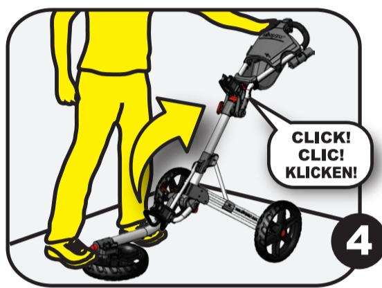
**Extend the handle up and forward until the wheels extend and the handle CLICKS into place.**
