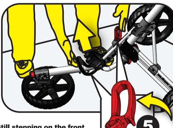
**Still stepping on the front wheel, pull up on the lower bag support and lock the main hinge LEVER.**
